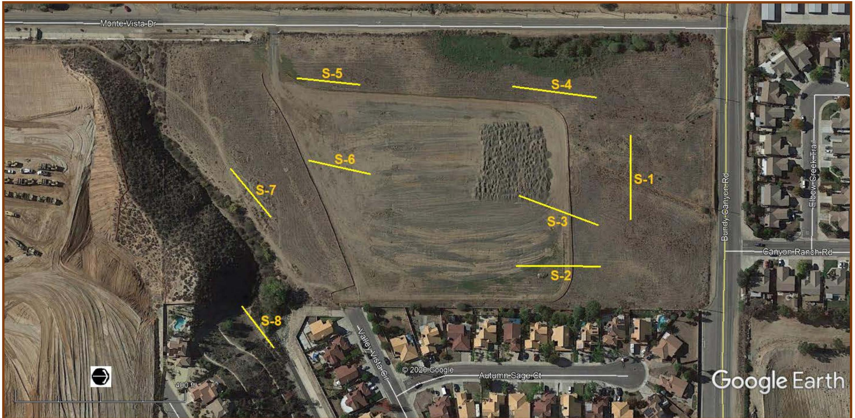
Google™ Earth (2020); Seismic survey lines (S-1 through S-7) shown as yellow lines.
