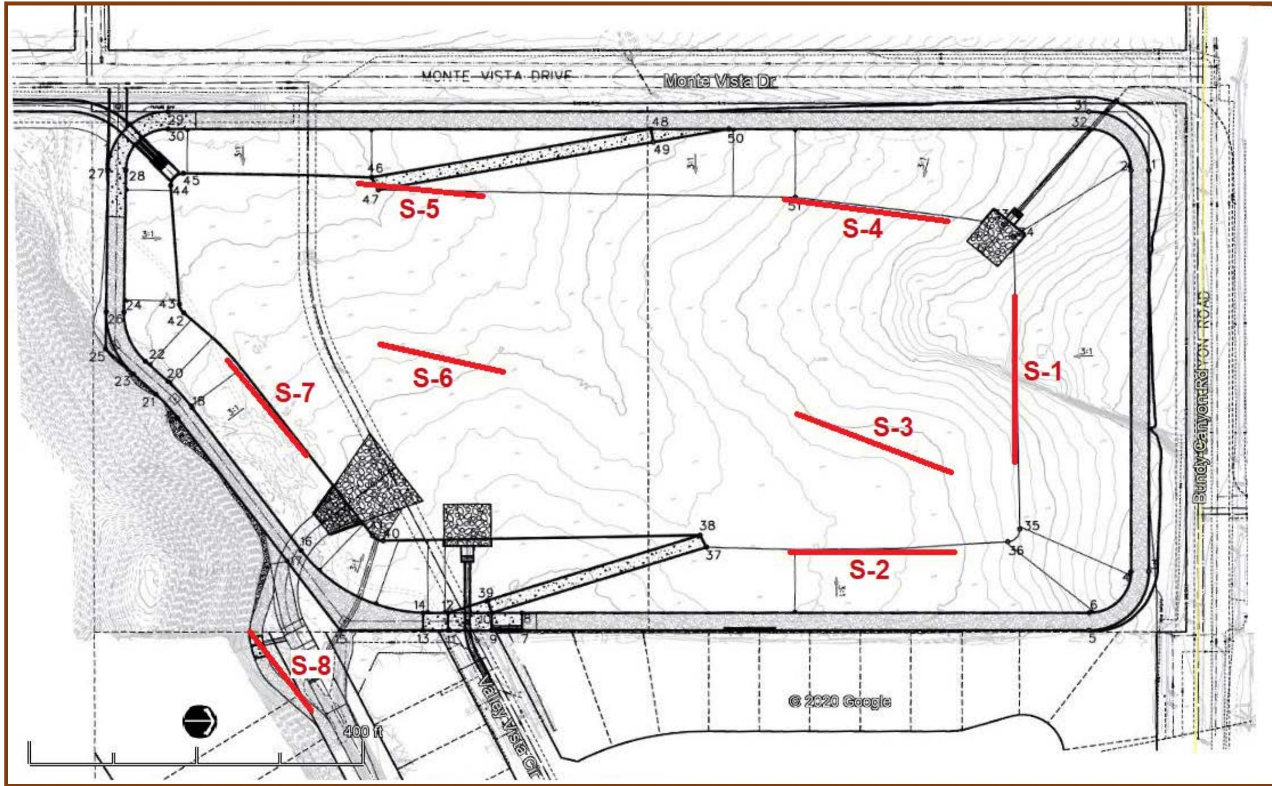
Base Map: RCFC Wildomar MDP Lateral 3, Stage 3 (Preliminary Sheet 5, partial copy); Seismic survey lines (S-1 through S-7) shown as red lines.
