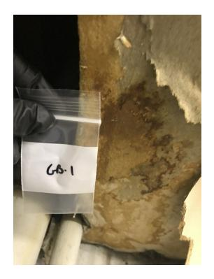
Picture 2: Ceiling gypsum board sampled was found to not contain asbestos
