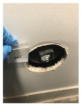
Picture 5: Gypsum board was sampled from the bathroom and showers
