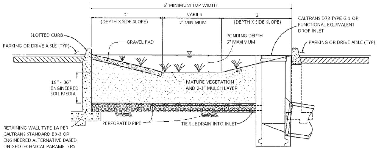
While the 18-inch minimum engineered soil media depth can be used in some cases, it is recommended to use 24 inches or a preferred 36 inches to provide an adequate root zone for the chosen plant palate. Such a design also provides for improved removal effectiveness for nutrients. The recommended ponding depth inside of a Bioretention Facility is 6 inches; measured from the flat bottom surface to the top of the water surface as shown in Figure 1.
